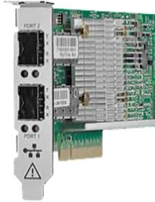
HPE StoreFabric CN1100R Dual Port Converged Network Adapter
