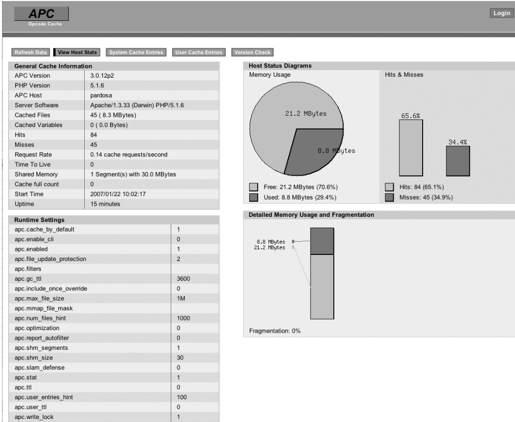
Figure 22-1. Alternative PHP Cache (APC) comes with an interface that displays memory allocation and the files currently within the cache.
